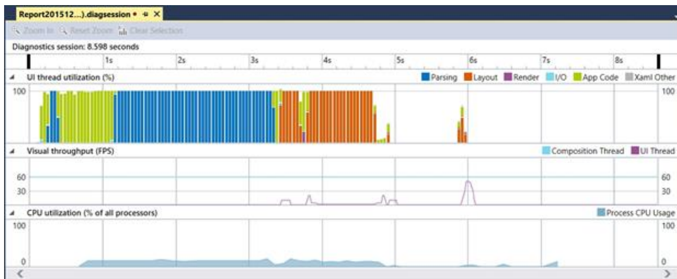
Figure 6: A recording of application startup with the timeline and CPU usage tools
